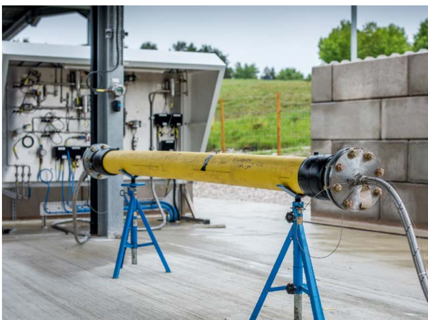
Figure 24. Hydrogen pipework under test. Image courtesy of Northern Gas Networks.
