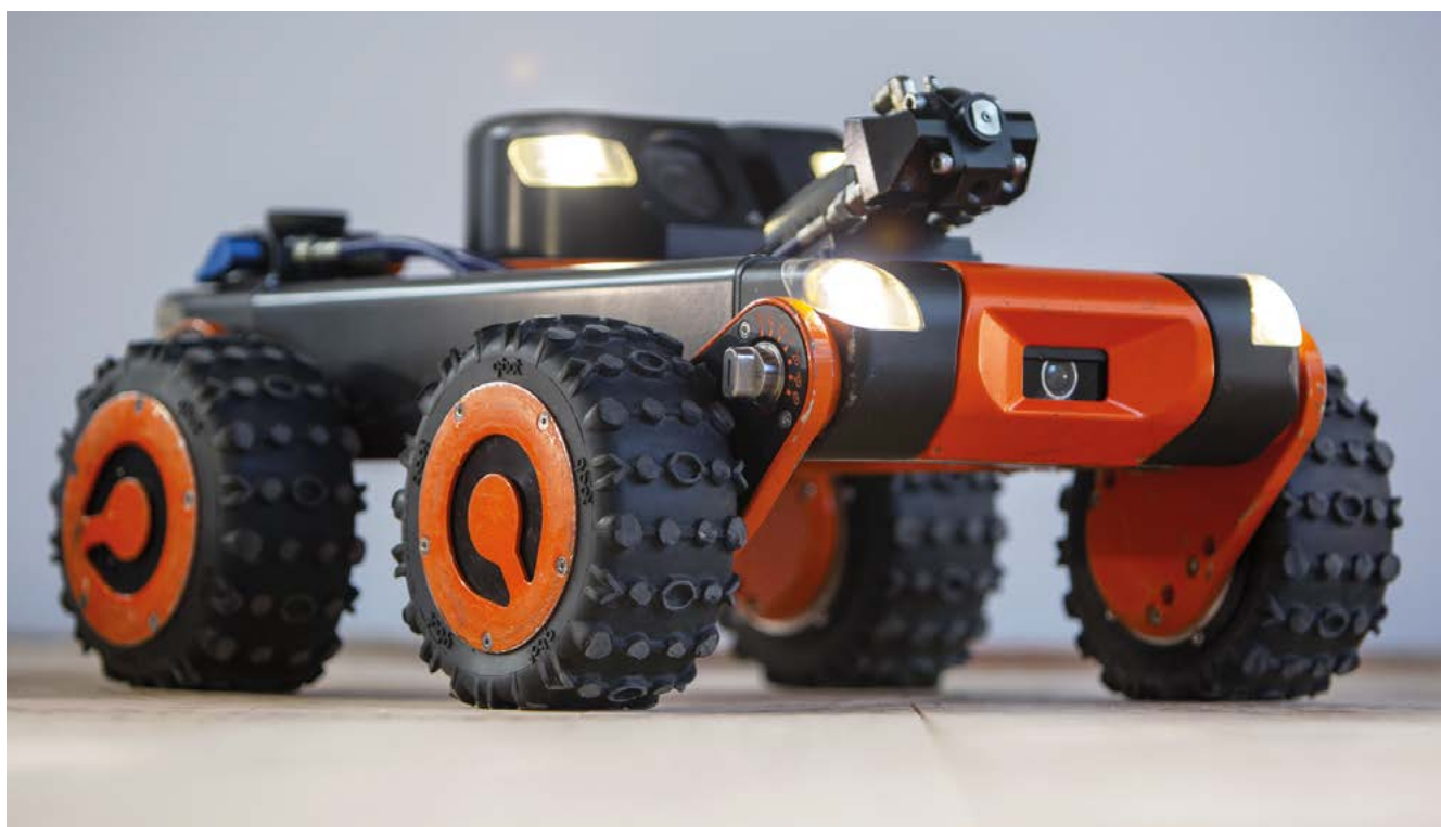
Figure 15. Q-Bots offer a new approach to insulating below floors, opening up an otherwise tiny market that has the scope to deliver significant energy savings in older buildings. Image courtesy of Q-Bots.
